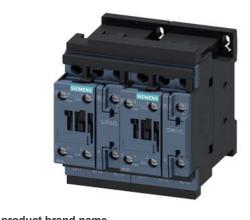
Reversing contactor assembly AC-3, 11 kW/400 V 110 V AC 50 Hz/120 V 60 Hz, 3-pole Size S0, screw terminal electrical and mechanical Interlock 2 NO integrated
