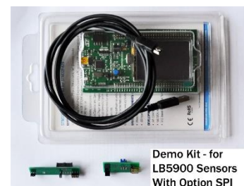
Demo Kit - for LB5900 Sensors With Option SPI SPI / I2C Demonstration Kit Available
