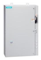
Non-reversing motor starter, Size 2, Three phase full voltage, Solid-state overload relay, OLR amp range 13-52A, 208VAC 60Hz coil, Combination type, 60A non-fusible disconnect, Enclosure NEMA type 4/12, Water/dust tight for outdoors, Extra-wide enclosure
