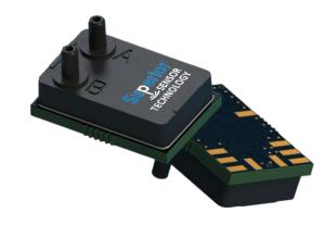
Industry leading accuracy - The ND Absolute Middle Pressure Series provides accuracy better than 0.10% FS and Total Error Band is also industry leading, typically better than 0.15% FSS.
