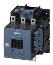
power contactor, AC-3 115 A, 55 kW / 400 V AC (50-60 Hz) / DC operation 96-127 V AC/DC auxiliary contacts 2 NO + 2 NC 3-pole, frame size S6 busbar connections drive: electronic with PLC interface 24 V DC spring-loaded terminal
