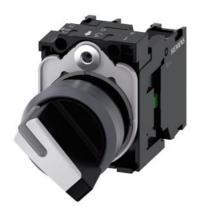
Selector switch, illuminable, 22 mm, round, plastic with metal front ring, white, selector switch, short, 2 switch positions O-I, latching, actuating angle 90°, 10:30h/13:30h, with holder, 1 NO, 1 NC, screw terminal, with laser labeling, lower case
