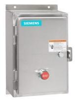
Non-reversing motor starter, Size 0, Three phase full voltage, Solid-state overload relay, OLR amp range 5.5-22A, 110V 50Hz / 120V 60Hz coil, Non-combination type, Encl. type 4X 304 S. Steel, Water/dust tight noncorrosive, Extra-wide enclosure
