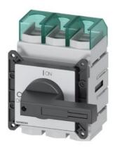
SENTRON, Switch disconnector 3LD, main switch, 3-pole, lu: 160 A, Operating power / at AC-23 A at 400 V: 75 kW, front-mounted, knob-operated mechanism, black, 4-hole mounting of the handle
