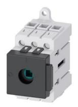
Load disconnector 3LD3, lu 63 A Main switch 3-pole Rated operating capacity at AC-23 A at 400V 22.0 kW Installation in distribution boards, Basic switch without Knob-operated mechanism
