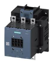
Power contactor, AC-3 185 A, 90 kW / 400 V AC (50-60 Hz) / DC operation 220-240 V UC without auxiliary contacts 3-pole, Size S6 Busbar connections Drive: conventional
