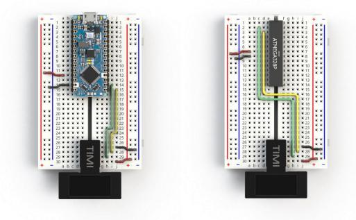
Note. Wiring simplified showing main wires only.
