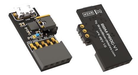
The BBM-PROG features a 3-pin jumper with shunt, which is present to change the way the programmer handles the Reset line, utilised by TIMI and other devices.
