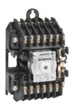
Mechanically held lighting contactor, Contactor amp rating 20A, 0 N.C. / 12 N.O. poles, Non-combination type, Enclosure NEMA type (open), No enclosure
