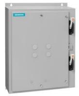
Duplex starter w/o alternator, Size 2, Three phase full voltage, Solid-state overload relay, OLR amp range 13-52A, 208VAC 60Hz coil, Combination type, Two 50A circuit breakers, Encl NEMA type 4X 304 S-Steel, Water/dust tight noncorrosive
