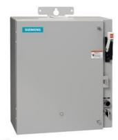
Pump control panel, Size 1, Three phase full voltage, Solid-state overload relay, OLR amp range 5.5-22A, 190-220/220-240V 50/60Hz coil, Standard type contactor, 30A fusible disconnect, 30A/250V fuse clip, HOA Sel Sw. <(>&<)> Start P.B., Enclosure NEMA type 3/3R, Weather proof outdoor use
