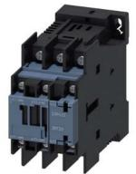
power contactor, AC-3 17 A, 7.5 kW / 400 V 1 NO + 1 NC, 24 V DC 3-pole, Size S0 ring cable lug connection
