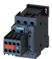
Power contactor, AC-3 32 A, 15 kW / 400 V 2 NO + 2 NC, 230 V AC 50/60 Hz, 3-pole Size S0, Screw terminal Captive auxiliary switch
