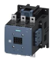
power contactor, AC-3 500 A, 250 kW / 400 V AC (50-60 Hz) / DC 110-127 V AC/DC auxiliary contacts 2 NO + 2 NC 3-pole, frame size S12 busbar connections drive: conventional spring-loaded terminal
