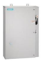
Non-reversing motor starter, Size 3, Three phase full voltage, Solid-state overload relay, OLR amp range 25-100A, Combination type, 100A fusible disconnect, 100A/250V fuse clip, Encl NEMA type 4X 304 S-Steel, Water/dust tight noncorrosive, Extra-wide enclosure
