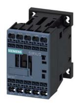
power contactor, AC-3 7 A, 3 kW / 400 V 1 NO, 24 V DC 0.7-1.25\* US, with diode integrated, 3-pole, size S00, spring-type terminal suitable for PLC outputs not expandable with auxiliary switch
