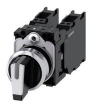
Selector switch, illuminable, 22 mm, round, metal, shiny, white, selector switch, short, 3 switch positions I>O<II, momentary contact type, actuating angle 2x45°, 10:30h/12h/13:30h, with holder, 2x1NO+1NC, Spring-type terminal
