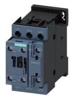
power contactor, AC-3 12 A, 5.5 kW / 400 V 1 NO + 1 NC, 200 V AC, 50 Hz 200-220 V, 60 Hz, 3-pole Size S0, screw terminal
