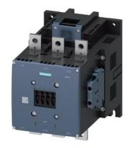
Contactor, AC-1, 690 A/690 V/40  $^{\circ}$ C, S12, 3-pole, 220-240 V AC/DC, with varistor, 2 NO+2 NC, Connection rail/ screw terminal
