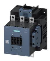
power contactor, AC-3 185 A, 90 kW / 400 V AC (50-60 Hz) / DC operation 380-420 V AC/DC auxiliary contacts 2 NO + 2 NC 3-pole, frame size S6 busbar connections drive: conventional screw terminal
