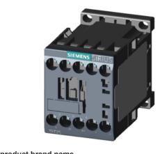
Power contactor, AC-3 12 A, 5.5 kW / 400 V 2 NO + 2 NC 220 V DC, 50 Hz 240 V, 60 Hz 4-pole Size S00 screw terminals
