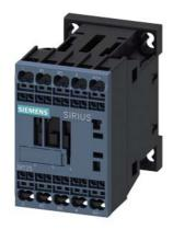
Power contactor, AC-3 12 A, 5.5 kW / 400 V 2 NO + 2 NC 110 V DC 4-pole Size S00 Spring-type terminals
