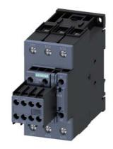
Power contactor, AC-3 80 A, 37 kW / 400 V 2 NO + 2 NC, 220 V AC 50/60 Hz, 3-pole Size S2, screw terminals
