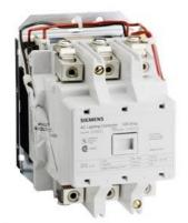
Mechanically held lighting contactor, Contactor amp rating 100A, 0 N.C. / 4 N.O. poles, 440VAC 50HZ/480VAC 60HZ coil, Non-combination type, Enclosure NEMA type (open), No enclosure
