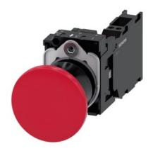
Mushroom pushbutton, 22 mm, round, plastic, red, 40mm, latching, pull-to-unlatch mechanism, with holder, 1 NO+1 NC, spring-type terminal, with laser labeling, upper case and lower case, always upper case at beginning of line
