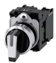
Selector switch, illuminable, 22 mm, round, metal, shiny, white, selector switch, short, 3 switch positions I>O<II, momentary contact type, actuating angle 2x45°, 10:30h/12h/13:30h, with holder, 1 NO, 1 NO, screw terminal
