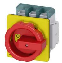
SENTRON, Switch disconnector 3LD, emergency switching-off switch, 3pole, lu: 100 A, operating power / at AC-23 A 400 V: 37 kW, front-mounted, 1 NC, 1 NO, rotary operating mechanism, Red / yellow, 4-hole mounting of the handle
