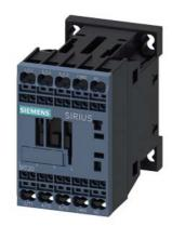
Power contactor, AC-3 7 A, 3 kW / 400 V 1 NO, 220 V AC, 50 Hz 240 V, 60 Hz, 3-pole, Size S00, Spring-type terminal
