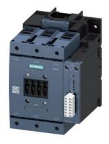
power contactor, AC-3 115 A, 55 kW / 400 V AC (50-60 Hz) / DC operation 96-127 V AC/DC auxiliary contacts 1 NO + 1 NC 3-pole, frame size S6 with box terminals drive: electronic with PLC / SIMOCODE - interface and remaining lifetime signal
