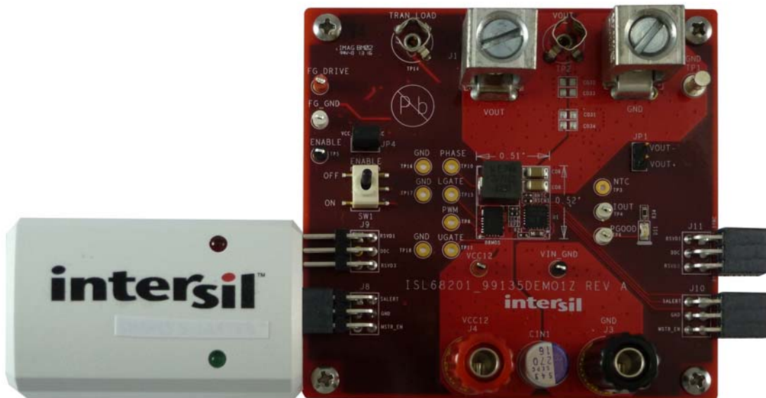
FIGURE 5. ISL68201-99135DEMO1Z DEMONSTRATION KIT SETUP
