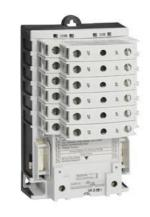
Electrically held lighting contactor, (convertible to mech. held), Amp rating 30A (tungsten 20A), 2 N.C. / 6 N.O. poles, 24V 60Hz / 20V 50Hz coil, Non-combination type, Enclosure NEMA type (open), No enclosure
