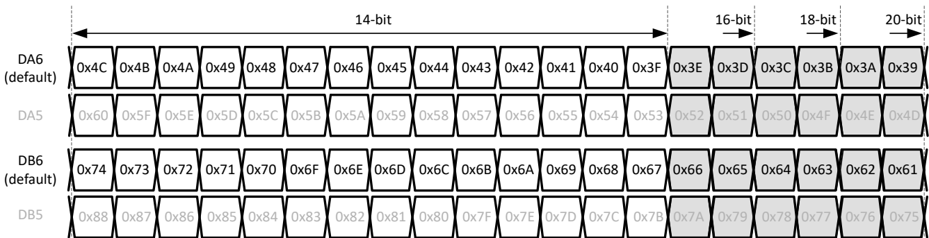
Figure 8-40. 1-wire output bit mapping
