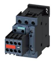
Power contactor, AC-3 25 A, 11 kW / 400 V 2 NO + 2 NC, 230 V AC, 50 / 60 Hz, with inserted varistor, 3-pole, Size S0 Screw terminal Captive auxiliary switch
