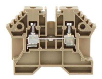
Feed-through terminal for direct mount/block variant, Screw connection, Mounting type: Mounting surface, Rated cross-section: 2.5 mm², Width: 5 mm, Colour: Beige
