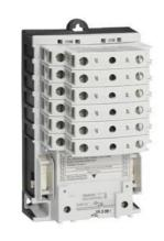
Electrically held lighting contactor, (convertible to mech. held), Amp rating 30A (tungsten 20A), 8 N.C. / 2 N.O. poles, 347V 60Hz coil, Non-combination type, Enclosure NEMA type (open), No enclosure
