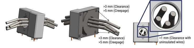
Reinforced insulation, insulation material group III, pollution degree 2, altitude < 5,000 m and overvoltage category II. Please take enough creepage distance between each pin.
