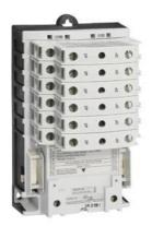
Electrically held lighting contactor, (convertible to mech. held), Amp rating 30A (tungsten 20A), 0 N.C. / 3 N.O. poles, 230-240V 60Hz/220V 50Hz coil, Non-combination type, Enclosure NEMA type (open), No enclosure
