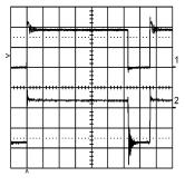
Trace 1: Drain of Q1 at Vin = 75VDC; Volts/div = 50.0V
