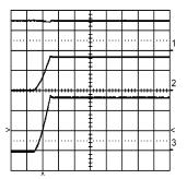
Trace 1: Input Voltage, at 30VDC. Volts/div = 20.0V Trace 2: Output Voltage, at 5% load. Volts/div = 2.0V Trace 3: Output Current, at 5% load. Amps/div = 100mA Horizontal Resolution = 1.0ms/div
