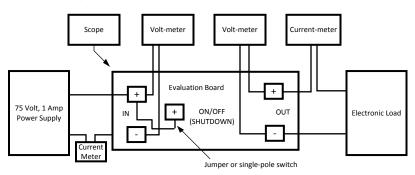
Figure 2. Typical Evaluation Setup
