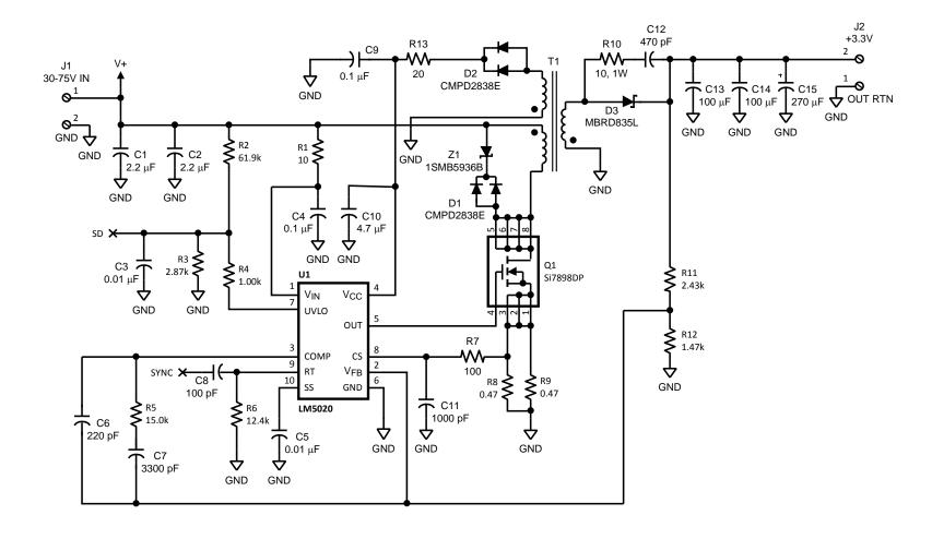
Figure 12. Application Circuit: Input 36V to 78V, Output 3.3V, 4.5A
