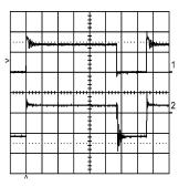
Trace 1: Drain of Q1 at Vin = 50VDC; Volts/div = 50.0V
