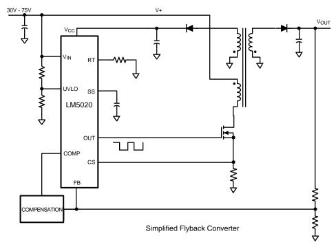
Figure 1. Simplified Flyback Converter
