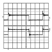
Trace 1: Drain of Q1 at Vin = 30VDC; Volts/div = 50.0V
