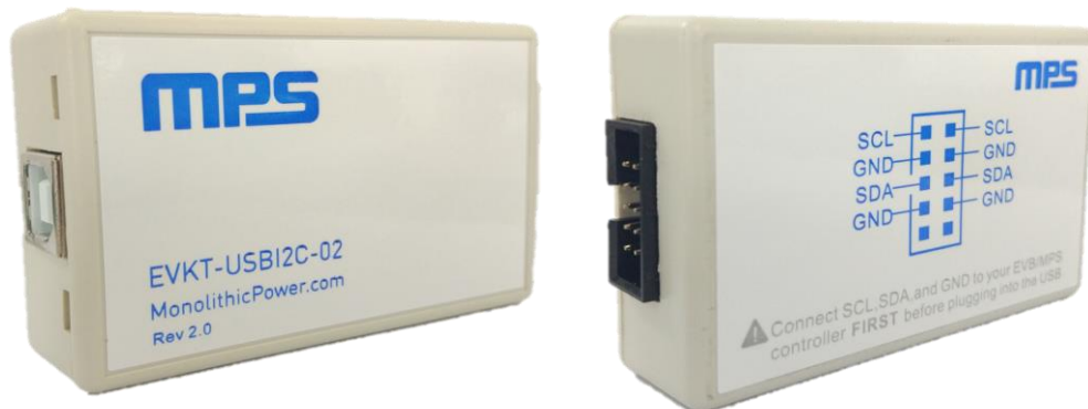
Figure 3: EVKT-USBI2C-02 Communication Interface
