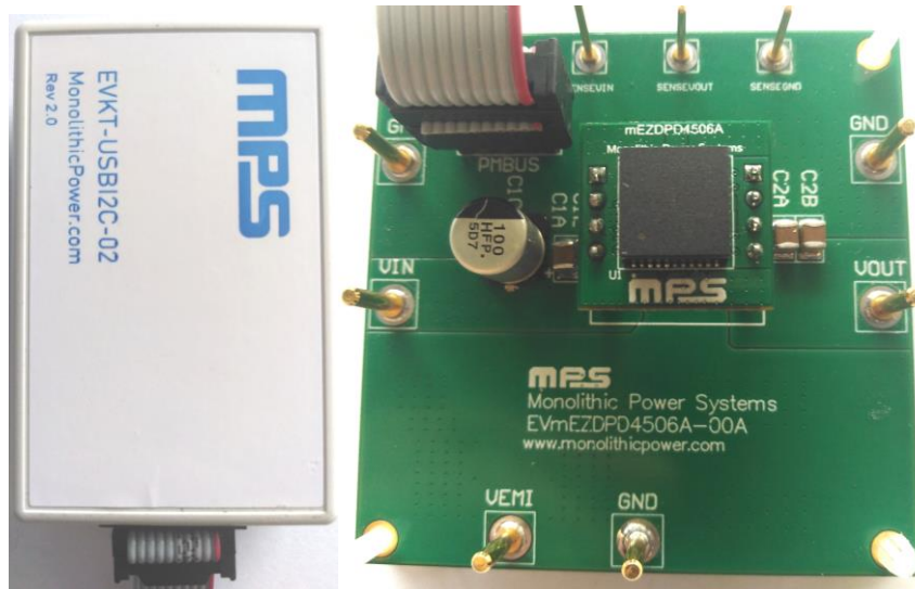
Figure 5: EVB to MPS I 2 C Communication Interface Device Wire Connection
