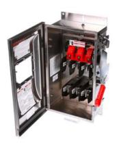
Siemens Low Voltage Circuit Protection Heavy Duty Safety Switches. Type: ENCLOSED, SAFETY SWITCH Std: CSA V. Rating: 600V A. Rating: 100A Wattage: 3W No. Of Poles: 3P F. Rating: 60Hz Action: SINGLE THROW Material: SS Enclosure: TYPE 4X. 2-3 point mounting holes. Insulation: YES O. Cycles: 10000 O. Temperature: (-20F-120F) AMBIENT TEMPERATURE Environmental Conditions: INDUSTRIAL CORROSIVE RESISTANCE
