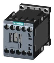
Power contactor, AC-3 9 A, 4 kW / 400 V 2 NO + 2 NC 48 V AC, 50/60 Hz 4-pole Size S00 Screw terminal
