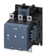
vacuum contactor, AC-3 300 A, 160 kW / 400 V, AC (50-60 Hz) / DC operation 240-277 V AC/DC auxiliary contacts 2 NO + 2 NC 3-pole, frame size S10 busbar connections drive: conventional
