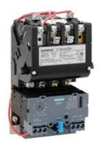
Non-reversing motor starter Size 0 Three phase full voltage Solid-state overload relay OLRelay amp range 3-12A 380-440/440-480V 50/60HZ coil Combination type No enclosure
