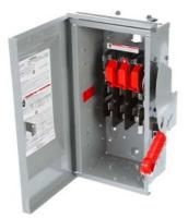
Siemens Low Voltage Circuit Protection Heavy Duty Safety Switches. Type: ENCLOSED, SAFETY SWITCH Std: UL V. Rating: 240V A. Rating: 30 A Wattage: 4W No. Of Poles: 3P F. Rating: 60Hz Action: SINGLE THROW Material: 304SS Enclosure: TYPE 3R. 2-3 point mounting holes. O. Cycles: 10000 O. Temperature: (-20F-120F) AMBIENT TEMPERATURE Environmental Conditions: OUTDOOR
