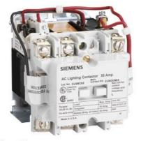
Mechanically held lighting contactor, Contactor amp rating 30A, 0 N.C. / 2 N.O. poles, 208VAC 60HZ coil, Non-combination type, Enclosure NEMA type (open), No enclosure
