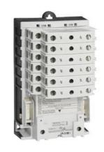
Electrically held lighting contactor, (convertible to mech. held), Amp rating 30A (tungsten 20A), 7 N.C. / 2 N.O. poles, 200-208V 60Hz coil, Non-combination type, Enclosure NEMA type (open), No enclosure
