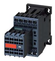
contactor relay, 4 NO + 4 NC, 24 V DC, size S00, spring-loaded terminal, captive auxiliary switch
